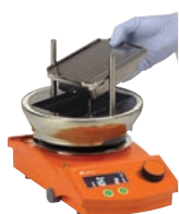
Insert the adapter into the GreenHouse base
