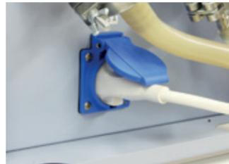
Socket for vacuum pump connection and control
