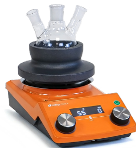
Carousel Core+ and Heat-On 500 ml block
