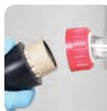
Insulated, 20mm bore vessel-to-manifold hoses are supported by the manifold and frame; minimising stress on the glass sidearms.
